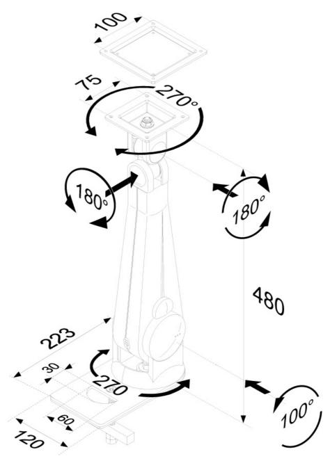
Neomounts Measuring unit: mm
