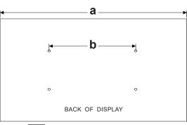
ENG Use the inside mounting holes when... a x 4 > 4098mm and a x 3 + b < 4064mm
