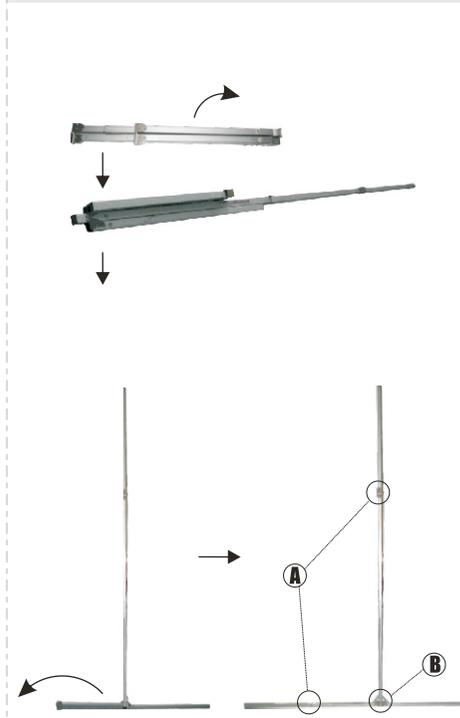
**4** Extend the leg support and screw it to the legs as shown.
