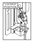
ENG OPTIONAL: Insert M5 x 10mm type-F socket pin screws to lock latches.
