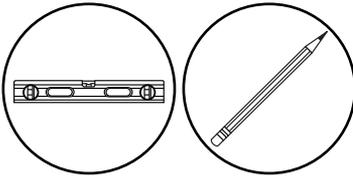
**ENG** Level wallplate. Mark mounting holes on stud center lines.
