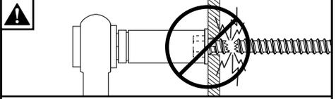
ENG Do not overtighten screws.
