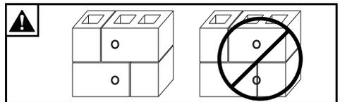
ENG Do not drill into mortar joints.
