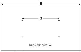
ENG Use the inside mounting holes when... a x 4 > 4098mm and a x 3 + b < 4064mm
