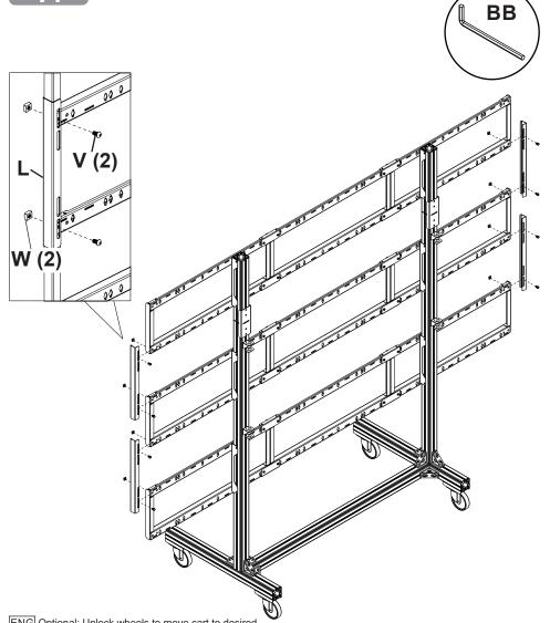
ENG Optional: Unlock wheels to move cart to desired location; Lock wheels before hanging screens.
