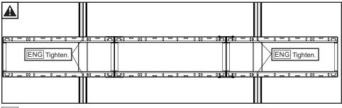
ENG Cross supports must center on vertical leg supports.
