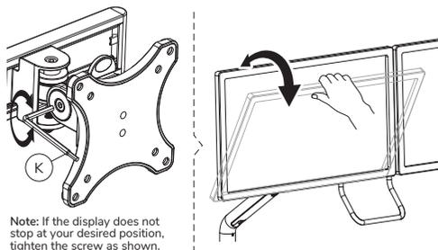
Note: If the display does not stop at your desired position, tighten the screw as shown.
